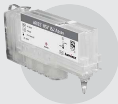
Step 1 Load the sample into the cassette
