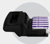
Step 3 Insert up to six cassettes into the magazine
